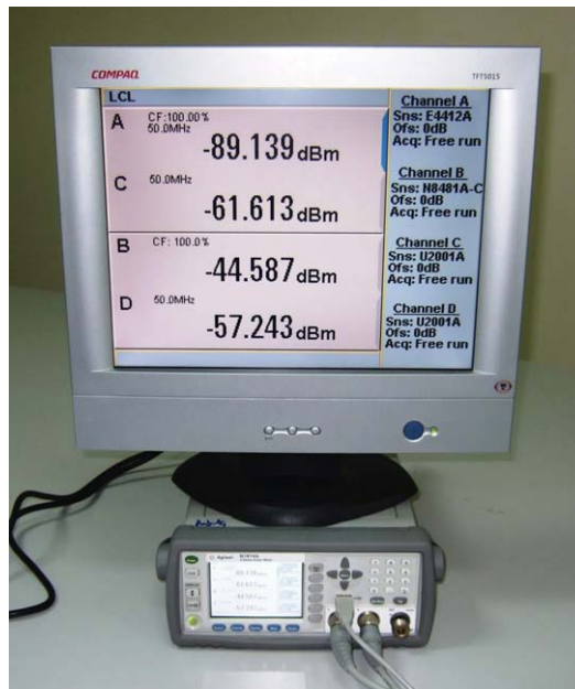
Figure 16. The N1913/1914A's VGA output display on external monitor
