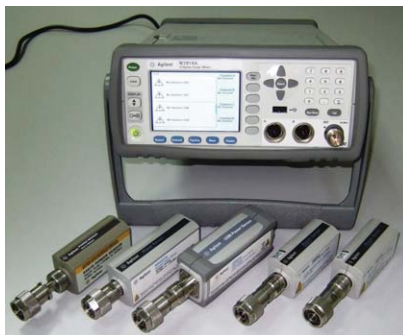
Figure 3. The Agilent 848x, N848x, E930x, E441x, and U2000 Series USB power sensors that are supported by the N1913/1914A
